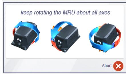
Figure 52 - The MRU must be rotated for the software to keep collecting calibration data.
